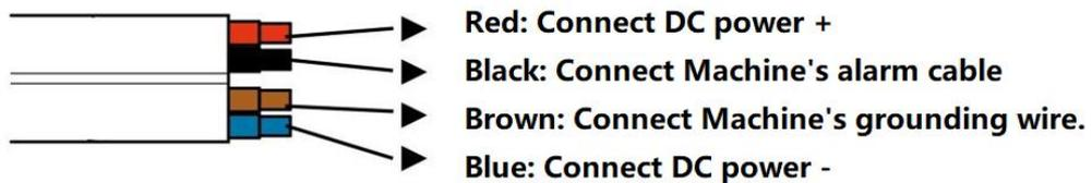
*Switch on power after cables are connected according to the guidance in above picture.*
