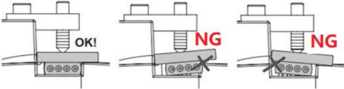
*The resistances are more than 10KΩ when cables connect with pins correctly.*
